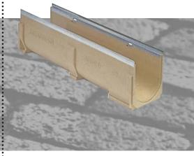
Opening width: 100 mm **Channel width:** 130 mm **Channel height:** from 150 mm
